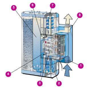
Compressed air is led through the inlet of the dryer (1) and across the prefilter (2).
